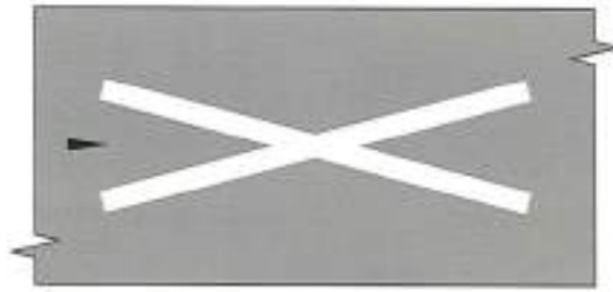
WM1 - RAILWAY CROSSING AHEAD
